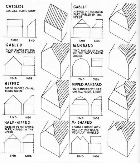
FIG. 22. Types of Roof Formation.
