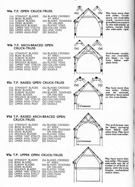
FIG. 14. VI. Through-Purlin Open Trusses.
