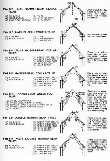
FIG. 10. IV. Butt-Purlin Hammer-Beam Trusses.
