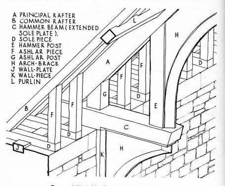
FIG. 7. Ashlaring: Butt-Purlin Hammer-Beam Truss.
