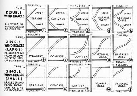
FIG. 18. Types of Wind-Brace (From Trusses to Side-Purlins, Wall-Plates, or Ridge-Purlins).
