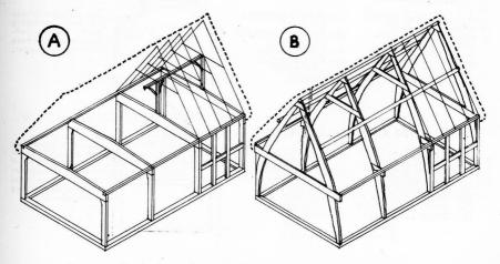
Comparison of Box-Frame and Cruck-Frame types of structure. FIG. 13.
