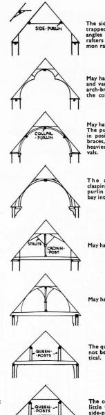
The side purlins are trapped between the angles of the collarrafters and the common rafters.
