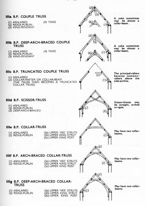
FIG. 8. III. Butt-Purlin Open Trusses.
